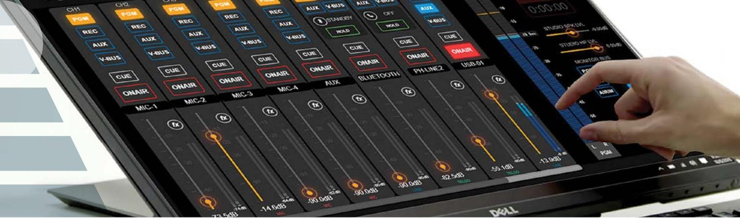
**All channels can be remotely controlled** from others studios via LAN or Internet, using a tablet or a PC computer. Using a touch screen video monitor you can build remote consoles without additional costs.
