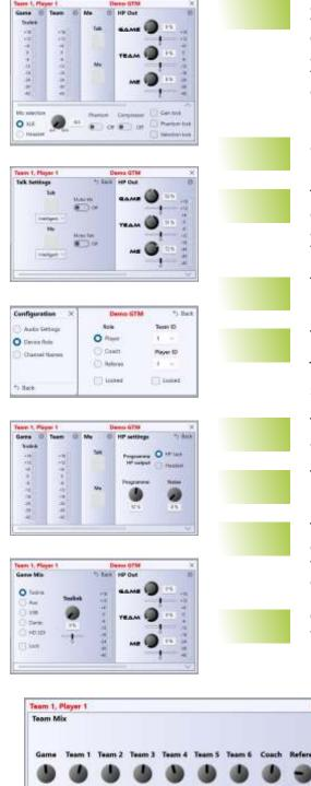
Adjust the incoming microphone gain via the XLR or headset connection. The Glensound Referee compressor is automatic and prevents clipping, but a further compressor can be added to level out the audio signal. A meter will show real time input level.
