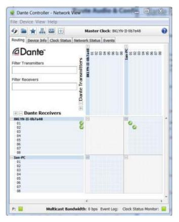
identify and resolve any potential network issues. You can also quickly and easily backup, restore, move, and reuse Dante network configurations using Presets, and edit Dante routing configurations offline.
