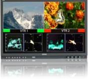
More than one signal may be monitored at once with PiP (Picture-in-Picture) and PbP (Picture-by-Picture) functions. PbP displays two inputs side by side in original aspect ratio, full screen and half of each input.
